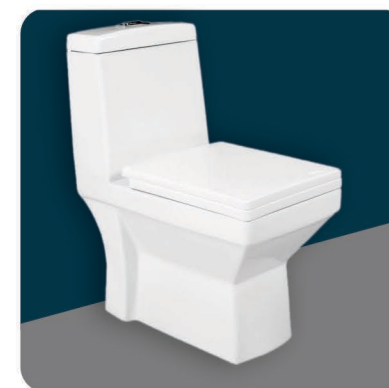
008 One Piece Closet Size : W 370 L 660 H 740mm S" Trap - 225mm (9") , 300mm (12")
