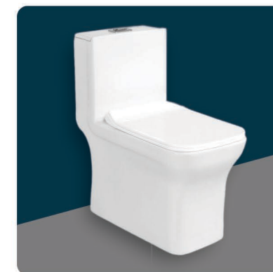
010 One Piece Closet Size : W 365 L 655 H 720mm S" Trap - 225mm (9") , 300mm (12")
